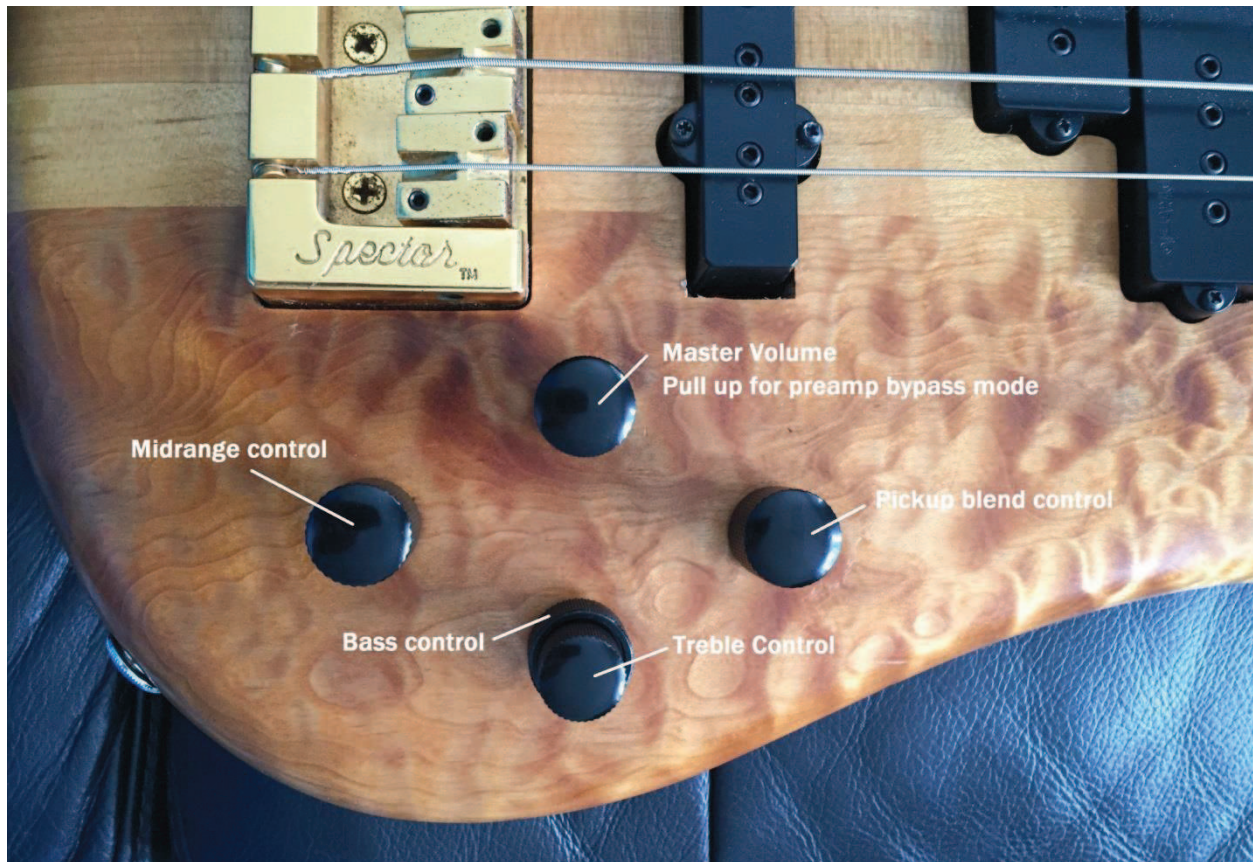
Figure 14: Knob installation and control functions
