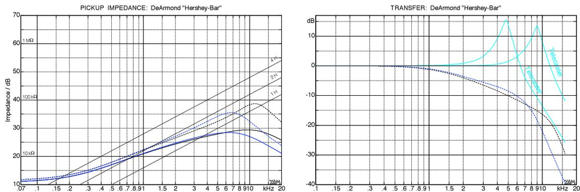
**Fig. 5.4.49:** DeArmond "Hershey-Bar". Left: impedance frequency response, w/out load and w/330 pF load. Loaded w/original 50-k $\Omega$ -potentiometer (—); w/out potentiometer (----). Right: transfer-frequency-response; Telecaster-bridge-pickup fro comparison (330 pF, 0 pF).
