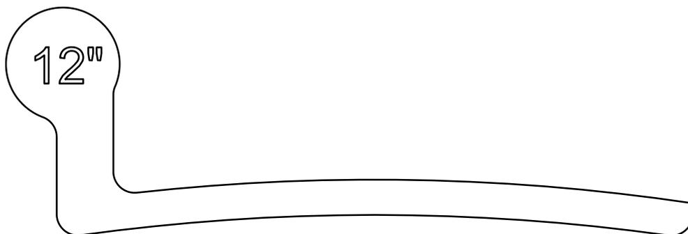
**Fig. 1** Example of a **Type A** template for a 12" curvature
