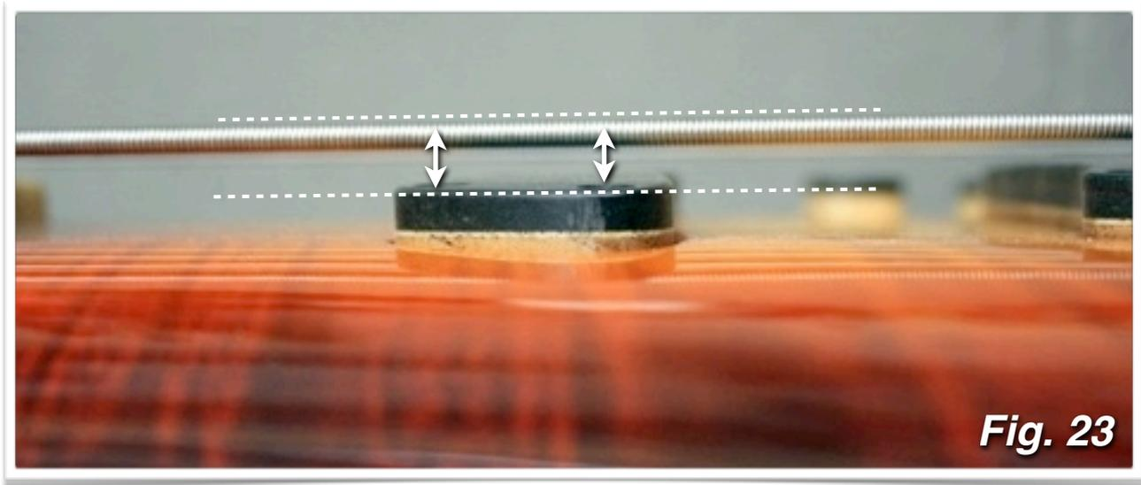
Lastly, if the pickups of your bass have more than 2 mounting screws, like those of the MusicMan® bass, which have 3 or the JazzBass®, which have 4, you will need to adjust the surface of the pickup so that it is parallel to the central axis of the string (**Fig. 23**).
