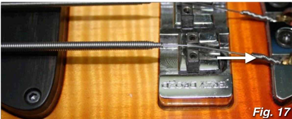
*The higher the pitch at the 12<sup>th</sup> fret in relation to the harmonic, the more you will have to move the saddle outward and away from the pickups to lengthen the string. Move the saddle away from the pickups if the note is higher than the harmonic.*
