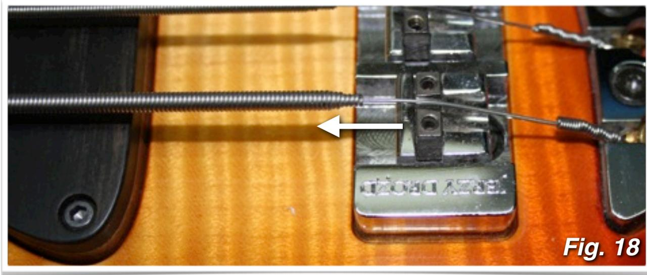
*The lower the pitch at the 12<sup>th</sup> fret in relation to the harmonic, the more you will have to move the saddle toward the pickups to shorten the string. Move the saddle toward the pickups if the note is lower than the harmonic.*
