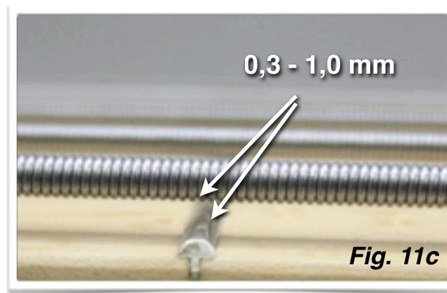
If the string doesn't touch the 7<sup>th</sup> through the 9<sup>th</sup> frets and there is some distance between the two, this means that there is an arc. Now, all we have to do is measure this distance to find out if it is correct.
