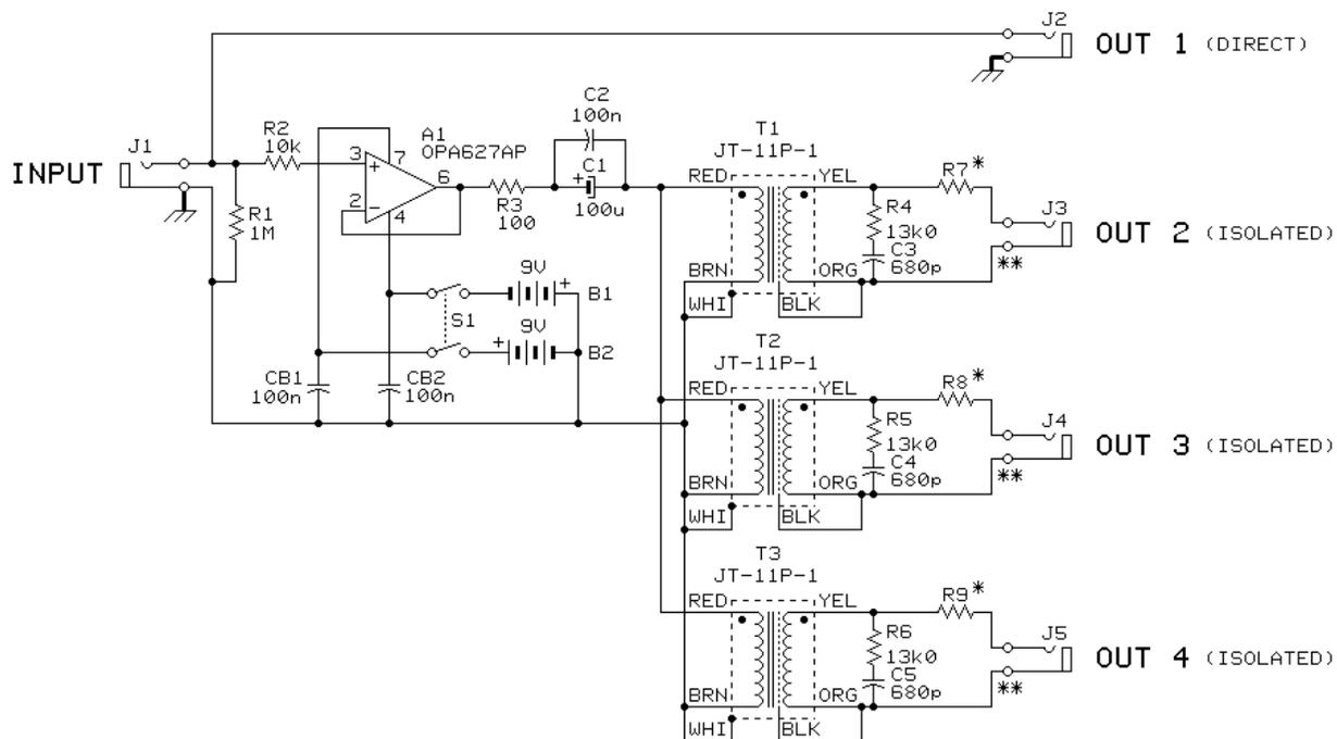
A LOWER COST OP-AMP, SUCH AS THE LF356N, MAY BE SUBSTITUTED FOR A1. ITS SLIGHTLY HIGHER NOISE (HISS) WILL BE INSIGNIFICANT UNLESS THE DC RESISTANCE OF THE PICKUP IS UNDER 3 kΩ,
