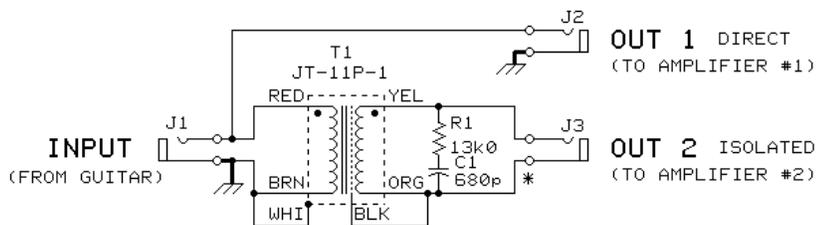
\* J3 MOUNTING MUST INSULATE IT FROM CHASSIS.
