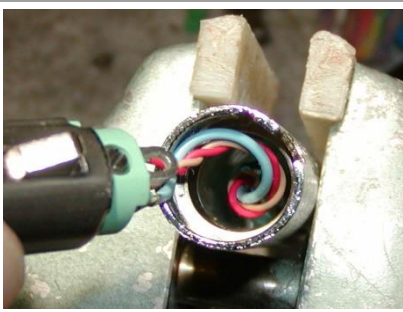
Inserting the female connector insert into the
