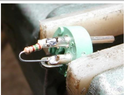
150-ohm resistor (R2) soldered across pin 2 and pin 3 of the male connector.
